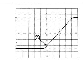
The 10% point on the waveform intersects the center vertical graticule line.
