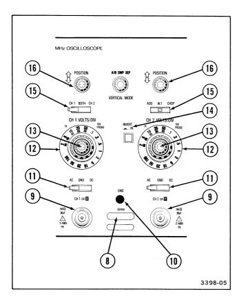
Figure 4. Vertical controls and connectors.
