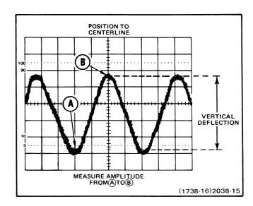
Figure 11. Peak-to-peak waveform voltage.
