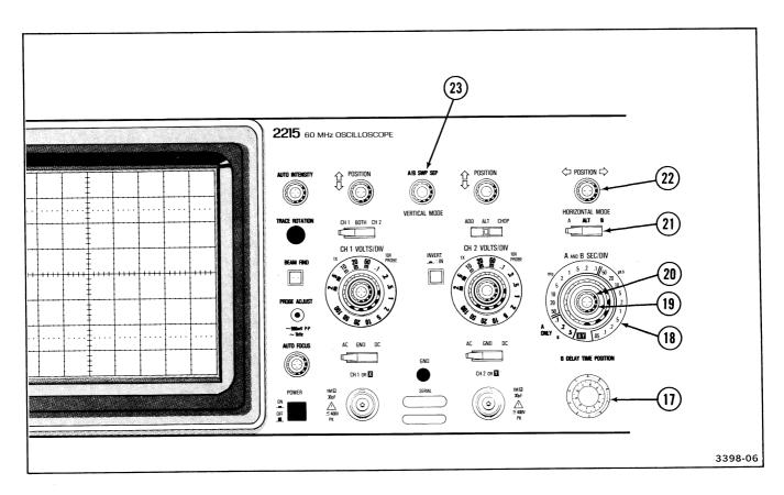
Figure 5. Horizontal controls.
