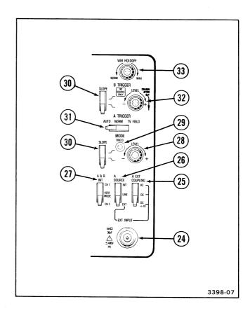
Figure 6. Trigger controls, connector, and indicator.
