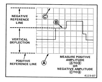
Figure 12. Instantaneous voltage measurement.
