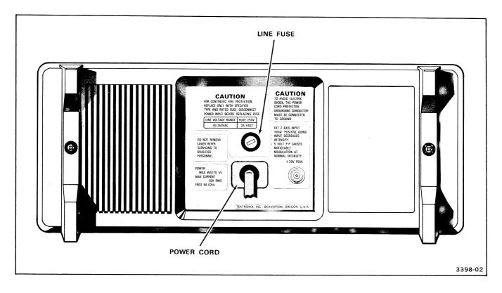
Figure 2. Line fuse and power cord.
