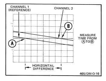
Figure 19. High-resolution phase difference.
