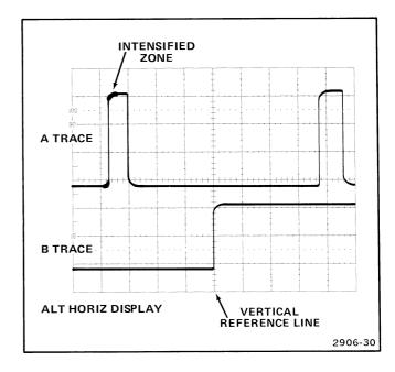
Figure 22. Time difference between repetitive pulses.
