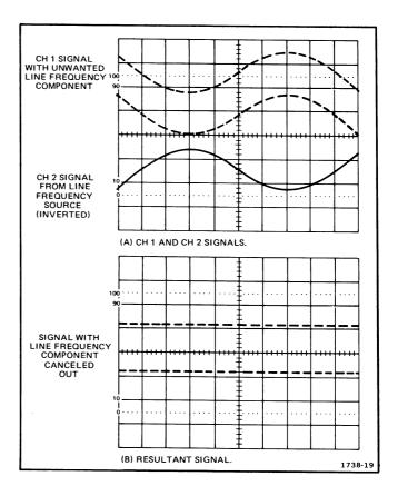
Figure 14. Common-mode rejection.
