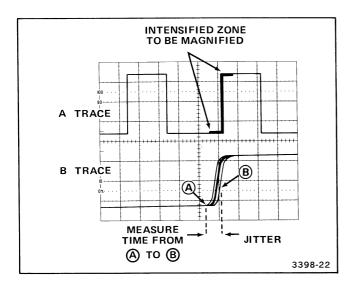
Figure 21. Pulse jitter.
