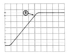
The 90% point on the waveform intersects the center vertical graticule line.
