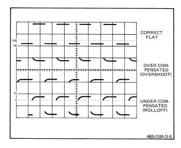
Figure 10. Probe compensation.
