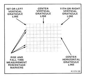
Figure 8. Graticule measurement markings.
