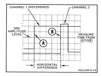
Figure 17. Time difference between two time-related pulses.
