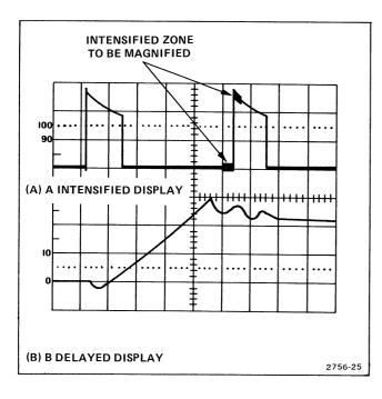
Figure 20. Delayed-sweep magnification.
